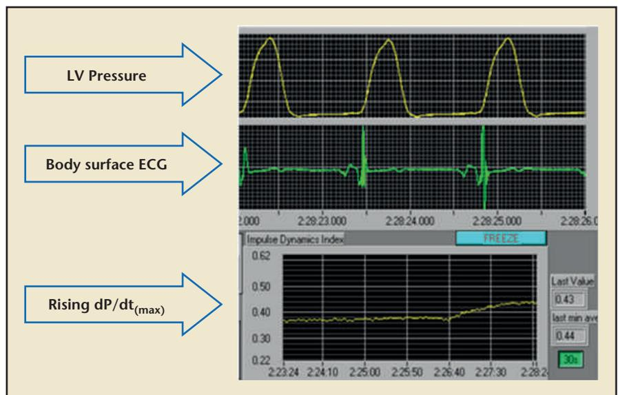
Figure 13.  $dP/dt_{max}$  display evaluation during OPTIMIZER™ IV, (Impulse Dynamics Inc., Orangeburg, NY) implant by the Monita system (Impulse Dynamics Inc.), indicating increase in contractility when CCM is active. CCM, cardiac contractility modulation;  $dP/dt_{max}$ , rate of left ventricle pressure rise in early systole; L, left ventricular.
