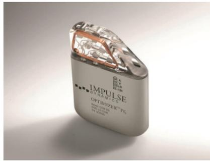
Figure 1. The OPTIMIZER™ IV<sub>s</sub> (Impulse Dynamics Inc., Orangeburg, NY) measures 60 × 47 mm and has a volume of 29 mL.
