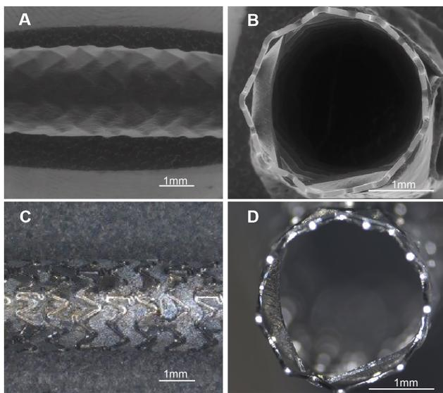
**Fig. 1. Microphotographs and digital photographs of covered stent.** (A) Microphotograph of overall covered stent (10 $\times$ ). (B) Microphotograph of cross-sectional covered stent (20 $\times$ ). (C) Digital photograph of overall covered stent (10 $\times$ ). (D) Digital photograph of cross-sectional covered stent (20 $\times$ ).
